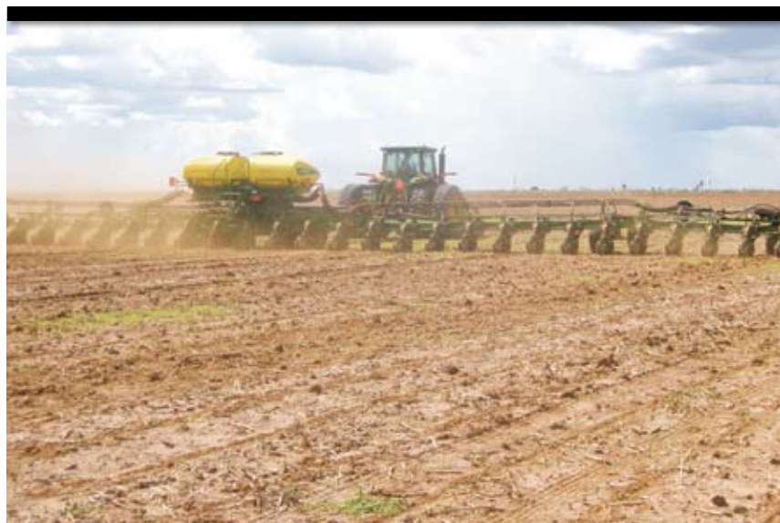
▲ Global Ag's new 108-ft., 36-row, 36-in. planter from Deere Bauer allows planting cotton at 84 acres/hour.
